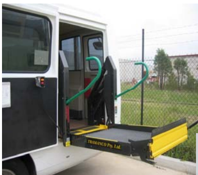
Side Loading Hoist
